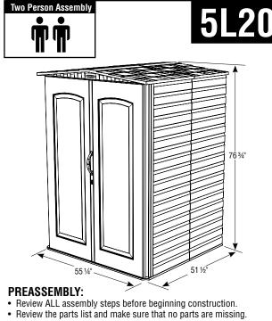
To simplify assembly and to ensure proper engagement of all components, apply a mild detergent to dovetail and snap fits before assembling.
